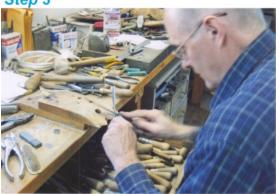
Step 3. Peter files excess silver from the forged piece. Files of various sizes and shapes are used, with varying rough and smooth surfaces.
