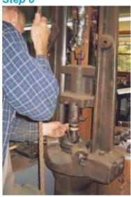
Step #8: Peter comples the process of shaping the bowl of the spoon with the drop hammer. The top piece is a special stake to fit the shape of that particular spoon. The bottom piece is a lead mold to fit the same shape.
