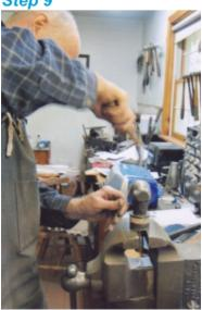
Step #9: Now he planishes the bowl of the spoon with a special stake and planishing hammer. This process removes any marks on the inside of the bowl and leaves hammer marks on the outside of the bowl.
