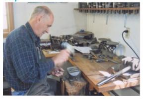
Step #1: Peter hammers the spoon into shape with a forging hammer on a special forging anvil
