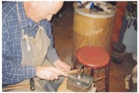
Step #2: Then, he "planishes" the spoon with special planishing hammers and anvil. Planishing is a process of refining the surface of the metal with highly-polished hammers
